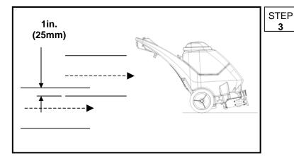
Push down on handle to raise vacuum shoe and brush before moving to the next cleaning pass. Overlap brush contact area approximately 1inch.
